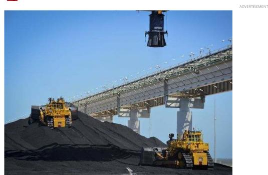
A week after the first load of coal arrives at the Wiggins Island Coal Export Terminal, dozers and trucks begin to move the coal to bed down the stockyard.
